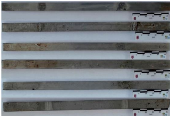
Figure 11. Bent steels right after SCC test.
