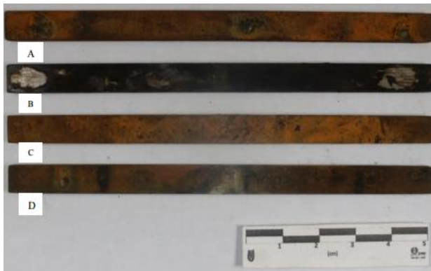
Figure 15. Steel A1 right after 3620 hours SCC test.
