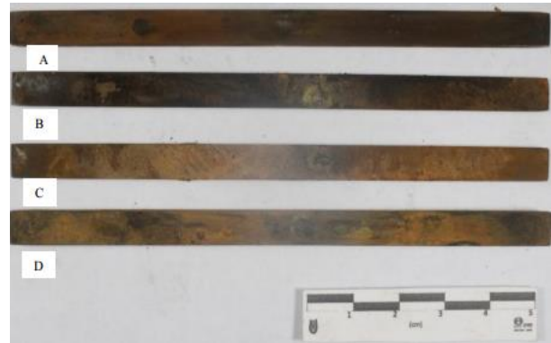
Figure 16. Steel A 3 right after 3620 hours SCC test.
